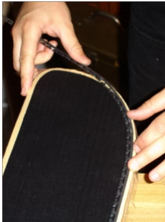
Figure 7. Bending steel edges around base.
