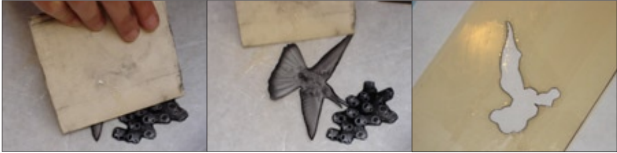
Figure 8. Graphics being laminated onto the underside of the topsheet.
