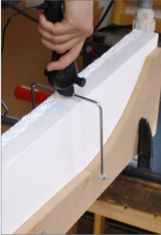
Figure 17. A foam cutter running along MDF jigs.
