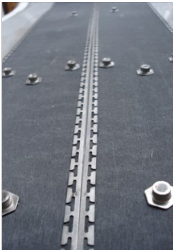
Figure 15. Some of the inserts are glued to the base.
