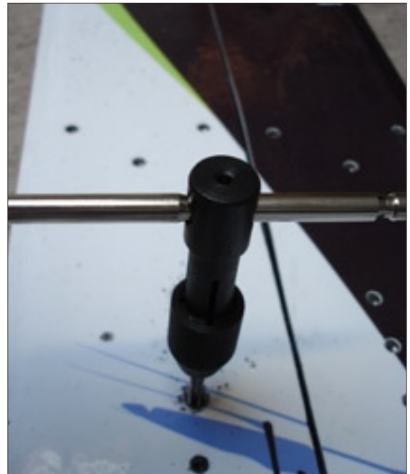
Figure 44. Tapping inserts on Wallowa board.
