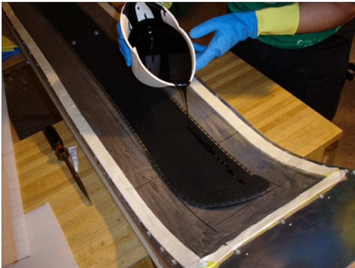
Figure 9. Lamination of the right half of the Float I board.
