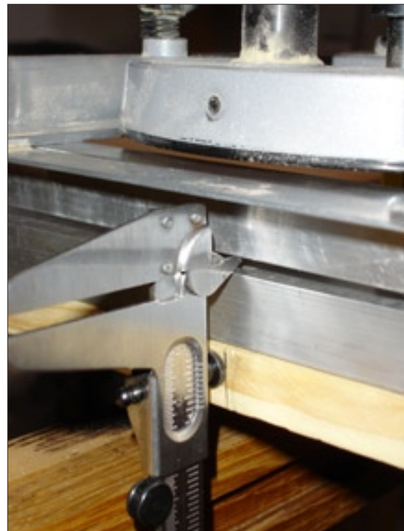
Figure 26. Vernier calipers and profiling tool.
