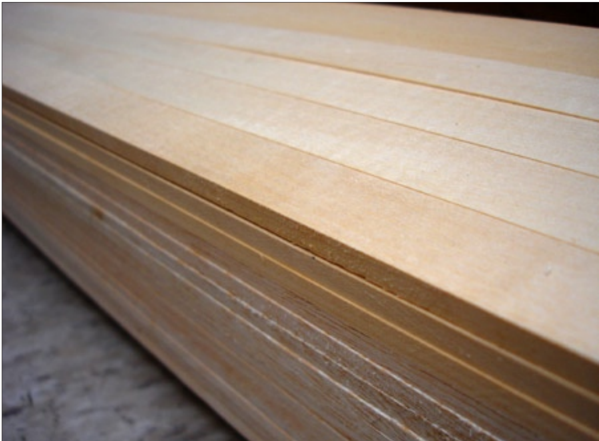
Figure 25. Balsa and basswood, bound to prevent warping.
